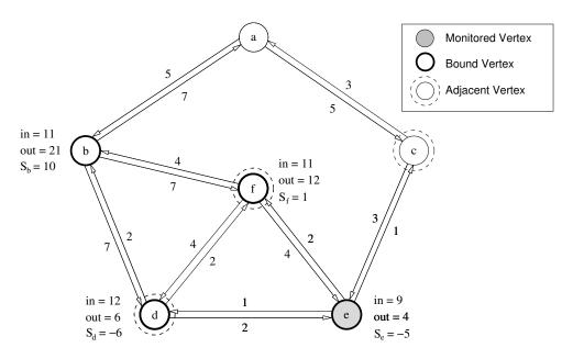
Figure 3.4: The final flow calculated on the graph for Example 1.
