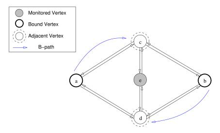
Figure 3.9: In this graph, we note that monitoring vertex e creates 2 disjoint B-paths; yet, the  $E_M$  matrix does not have linearly independent columns, and thus we cannot calculate the flow on the graph.
