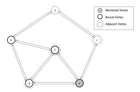
Figure 3.1: In this two-way directed graph, vertices b, d, e, and f are bound; vertices a and c are transport vertices. We put a sensor at vertex e, which gives the adjacent vertices to M as c, d, and f.
