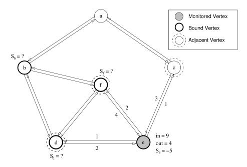
Figure 3.3: The graph from Figure 3.1, analyzed in Example 1. One can check that removal of the combined cutset  $C_M$  (shown in Figure 3.2) satisfies the conditions in Theorem 3.2.2, and we can calculate the flow everywhere in the graph (see Figure 3.4).
